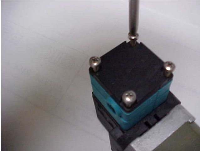
FIGURE 9 INSTALLATIONS OF COVER PLATE AND TIGHTENING OF SCREWS.
